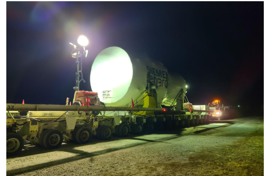
Siemens Energy Heavy Haul Gas Turbine #2
