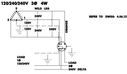
NOTE: MAXIMUM SINGLE PHASE LOAD IS LIMITED TO FIVE PER CENT OF THE TOTAL LOAD ON BANK
