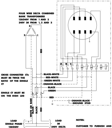
CUSTOMER TO FURNISH AND INSTALL "NATIONAL ELECTRICAL CODE" GRADE STEEL CABINET OF ADEQUATE SIZE FOR THE CURRENT TRANSFORMERS AND ALL WIRING CONNECTIONS
