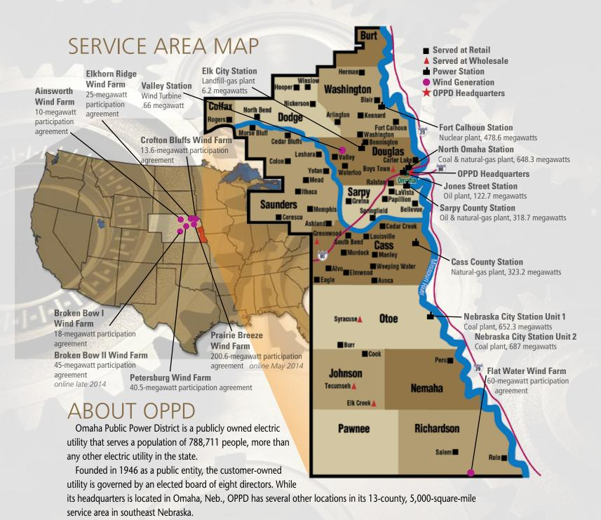
The majority of OPPD's power comes from three baseload power facilities: North Omaha Station and Nebraska City Station, both coal-fired, and Fort Calhoun Station, a nuclear power unit. Additional energy comes from three peaking units and renewable energy resources, including a landfill-gas unit and wind turbines.
