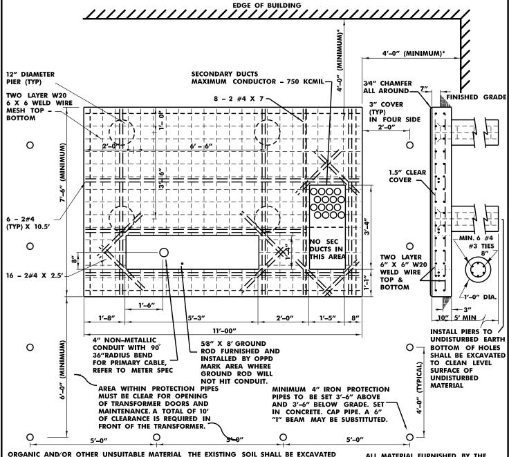
ORGANIC AND/OR OTHER UNSUITABLE MATERIAL SHALL BE REMOVED FROM SUBGRADE AND BACKFILL AREAS AND BACKFILLED WITH ACCEPTABLE GRANULAR FILL, COMPACTED TO 95 % OF MAXIMUM DENSITY AT OPTIMUM MOISTURE CONTENT ASTM D1557 AND D2049. IF THE TOP THREE (3) FEET OF SUBGRADE BENEATH THE SLAB IS SUSCEPTIBLE TO A HIGH WATER TABLE OR PERIODIC SATURATION,
