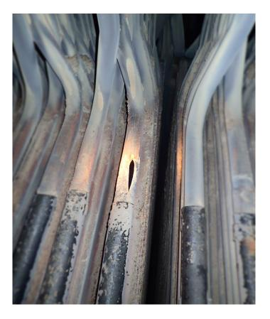
Reheat tube failures on NC2
