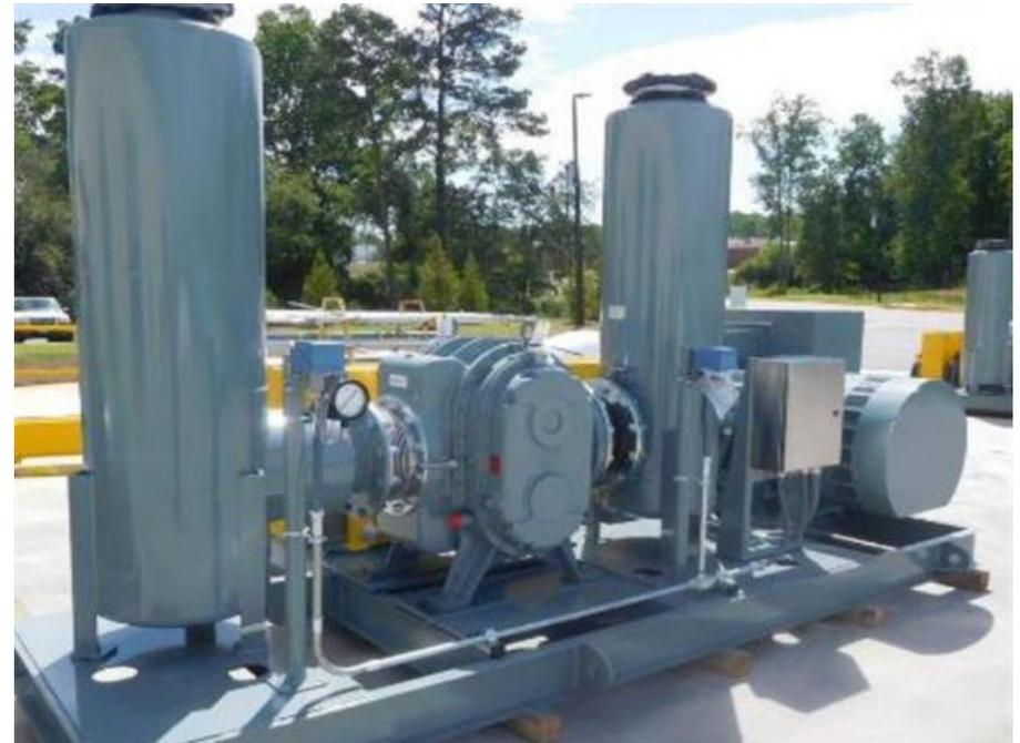
Example of new blower skid to pneumatically transfer ash
