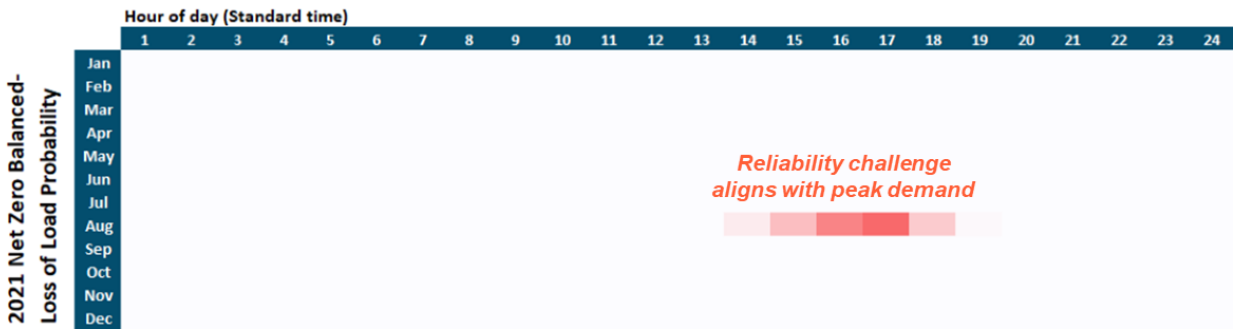
Figure 84. Loss-of-Load Probability Distribution by Month-Hour for the Net Zero Carbon Base Scenario in 2021
