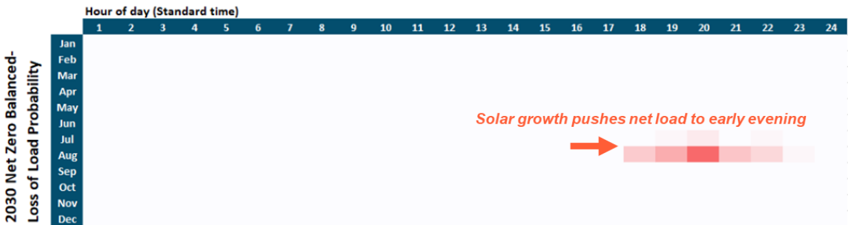
Figure 85. Loss-of-Load Probability Distribution by Month-Hour for the Net Zero Carbon Base Scenario in 2030
