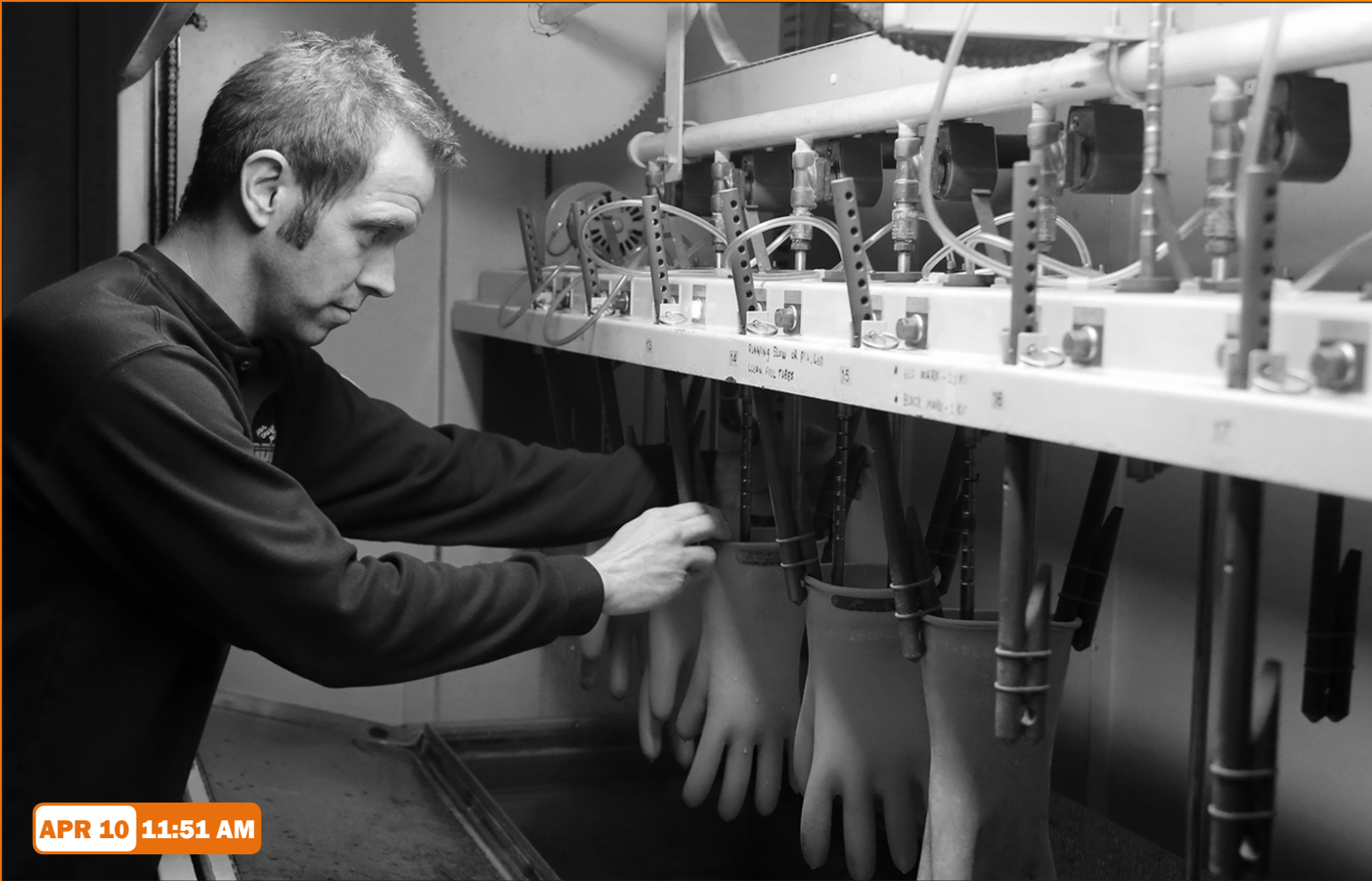
Maintenance worker Tyler Christensen tests all the gloves and other safety equipment used by OPPD's frontline workers.
